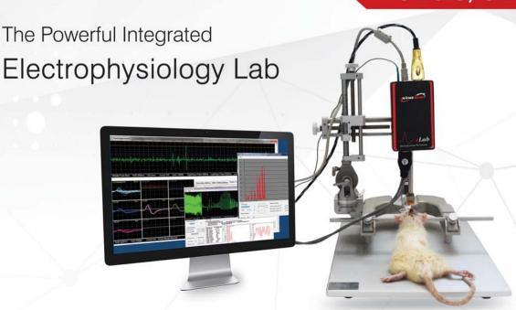
The integration of the eLab system with eProbe software is designed to record different classes of extracellular electrophysiological signals. Various devices and tools such as data acquisition, microelectrode amplifiers, ADC, stimulators, pulse generators, and window discriminators are integrated into one eLab system.
