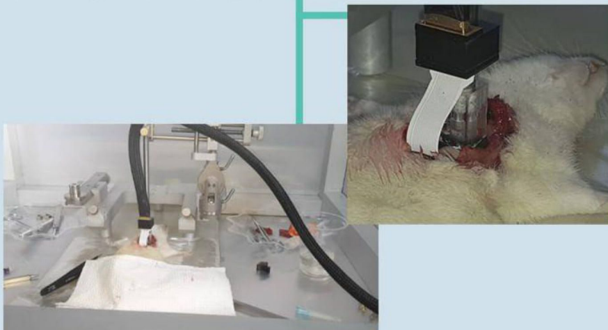
16 channels In-vivo ECG recording
